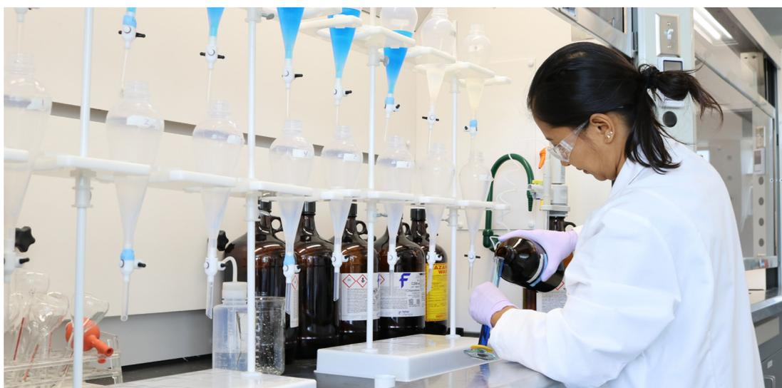
Quality Control Analyst performing Sufactants testing, a methane blue color reaction to detect the existence of anionic substances in water that may cause water corrosion or contamination.
